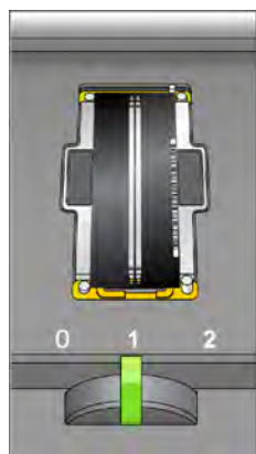
Figure 51 Flow Cell Lever in Position 1
