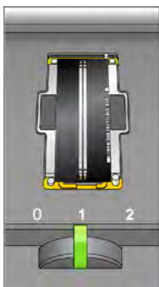
Figure 53 Flow Cell Lever in Position 1
