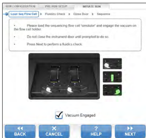
Figure 24 Load Seq Flow Cell Screen for a High Output Flow Cell
