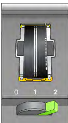
Figure 58 Flow Cell Lever in Position 2
