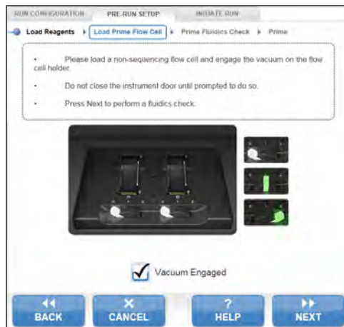
Figure 21 Load Prime Flow Cell Screen for High Output Flow Cells
