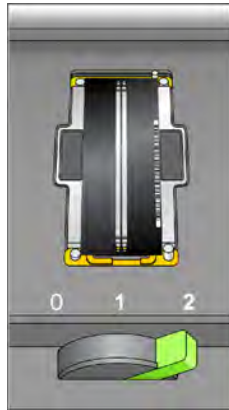
Figure 52 Flow Cell Lever in Position 2
