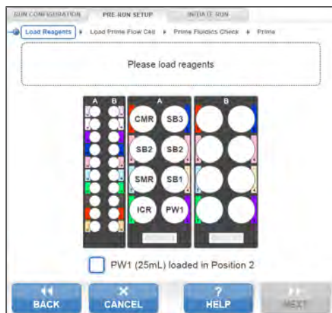
Figure 20 Load Reagents Screen for a High Output Flow Cell
